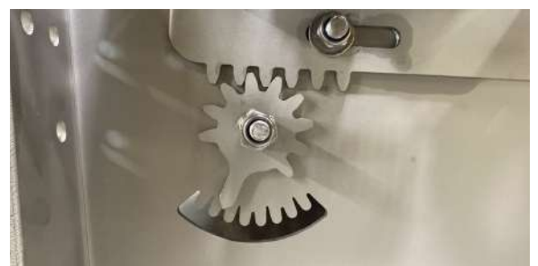
Clod roller gap adjustment moves all clod rollers equally with a single turn of the starwheel on each side (In store version)
