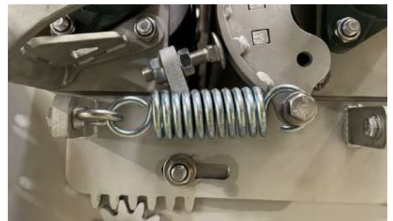
Clod roller gap adjustment moves all clod rollers equally with a single turn of the starwheel on each side (In store version)
