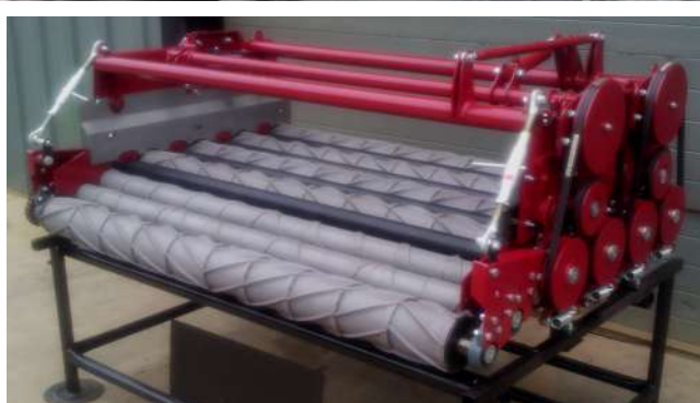
Mobile: hydraulic drive with Kevlar V belts
