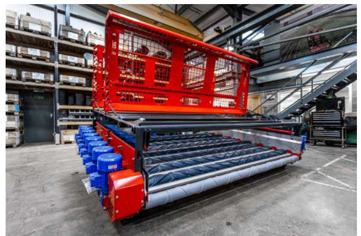
Gas strut operated top guard for easy access, supplied with magnetic safety switch (In store version)
