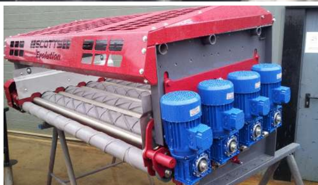
In store: direct electric motor drive
