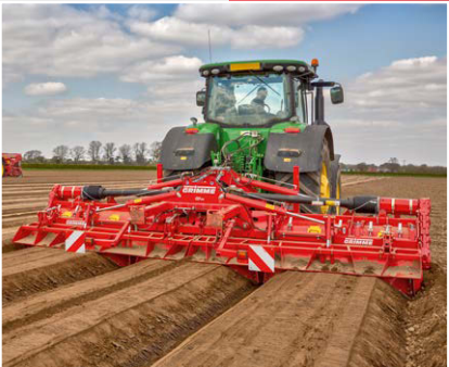
GF 600 6-row rotary tiller. for full width cultivation when planting vegetables or potatoes.
