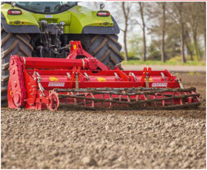
GF 400 4-row rotary tiller. for full width cultivation when planting vegetables or potatoes.
