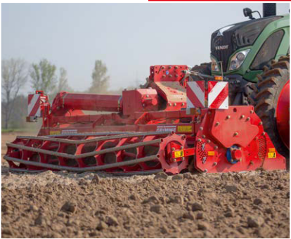
GR 300 / GR 360 Creates fine crumbled soil when cultivating on heavy soils.
