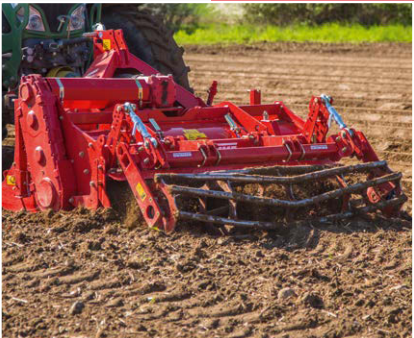
GF 200 2-row rotary tiller. for full width cultivation when planting vegetables or potatoes.
