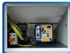
Frequency inverter with 3-phase thermal security
