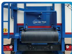
Aluminium slide with bearings and a plastic guide
