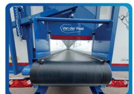
Endless welded conveyor belt
